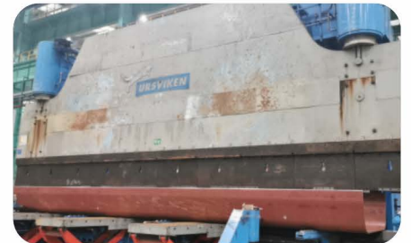
Bending Machine 15 MetersX 100mm Thickness
